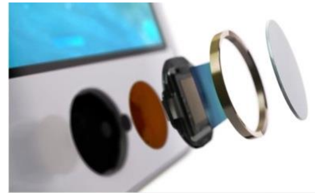
Apple's Touch ID Patent: Fingerprint Recognition Sensor
